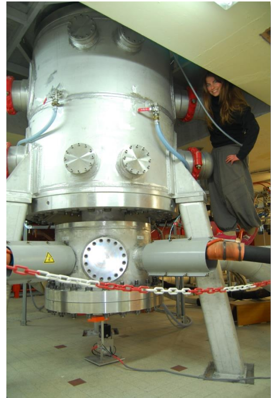
Water-cooled 35 T resistive magnet
