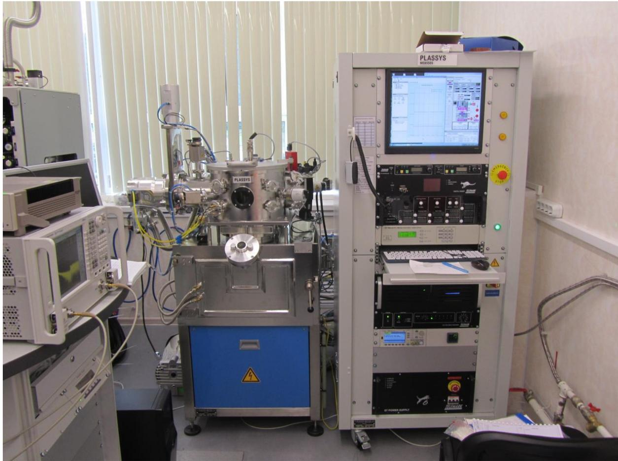
PLASSYS electron beam evaporation unit with load lock. The unit is dedicated for fabrication of Josephson junctions and was installed at RQC lab at ISSP Chernogolovka in June 2014
