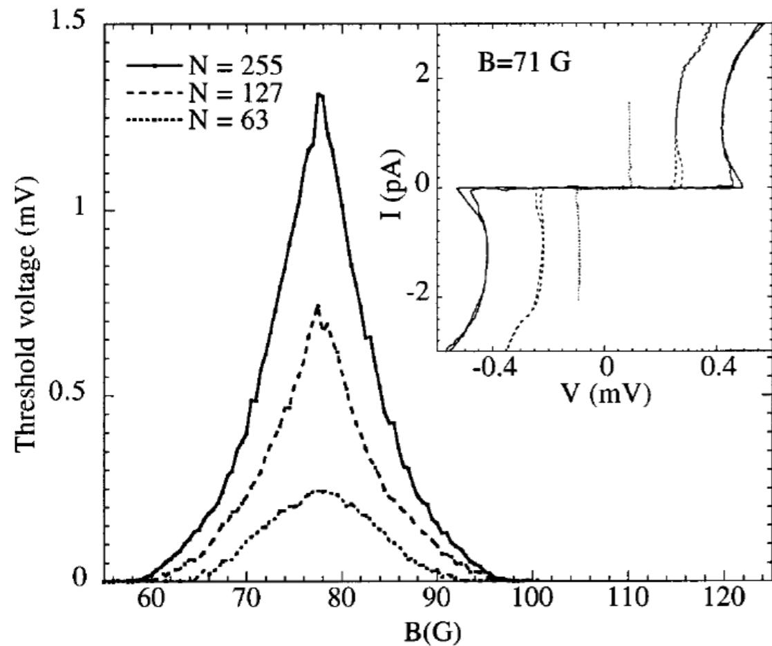
**Threshold voltage scales linearly with array length
